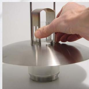
Inserting the smoke bell I.
