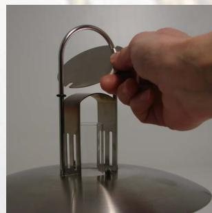
Inserting the smoke bell II. Pull down the 2 small o-rings along the handlebars to give room for the smoke bell. Insert the smoke bell in between the bars and let it rest on the 2 o-rings.
